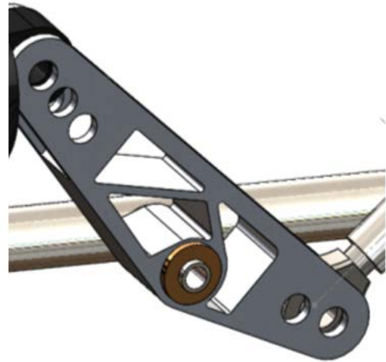
Figure 5: Real Life Example of Suspension Bell Crank [9]
